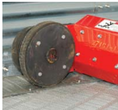
Solid rubber sweep drive wheel with 10:1 speed reduction minimizes wear on wheel and bin floor.
