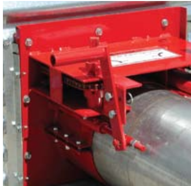
A simple shift mechanism is located outside of the bin to engage the sweep and to eliminate the need to enter the bin for sweep operation.
