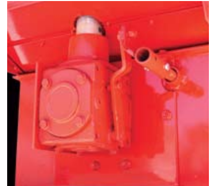
Sweep drive gearbox has internal shifting mechanism to engage sweep.
