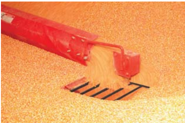
Heavy, high-angle sweep backboard construction.
