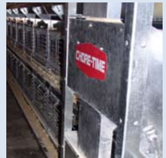
Traveling Hopper Feeder
